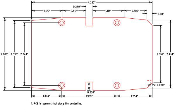
All solder pads are located on a 0.100" grid.
