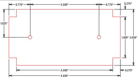
PCB is symmetrical in the X and Y directions.
