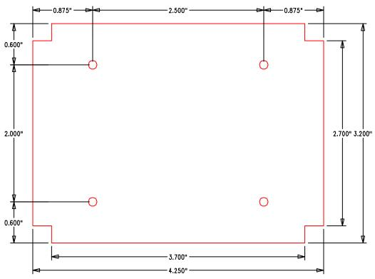
1. PCB is symmetrical in the X and Y directions.
