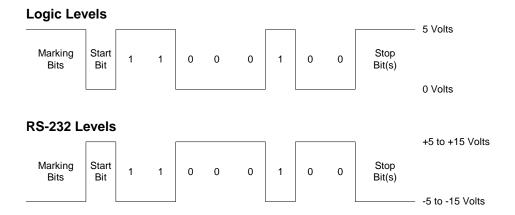
Figure 2 RS-232 Signal Levels
